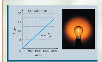
is  $8 \cdot 25 \cdot 7$  or 1400 watts. Use A = W/V to get A = 1400/ $120 \approx 11.7$ . So the lights will not blow a 15-amp fuse. See the accompanying figure.
